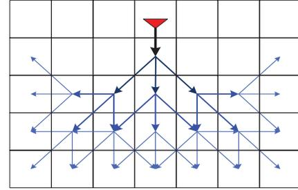
**Figure 3.** Agent's region of interest displayed as forward move projection span (possible paths) over a 3-step time horizon.
