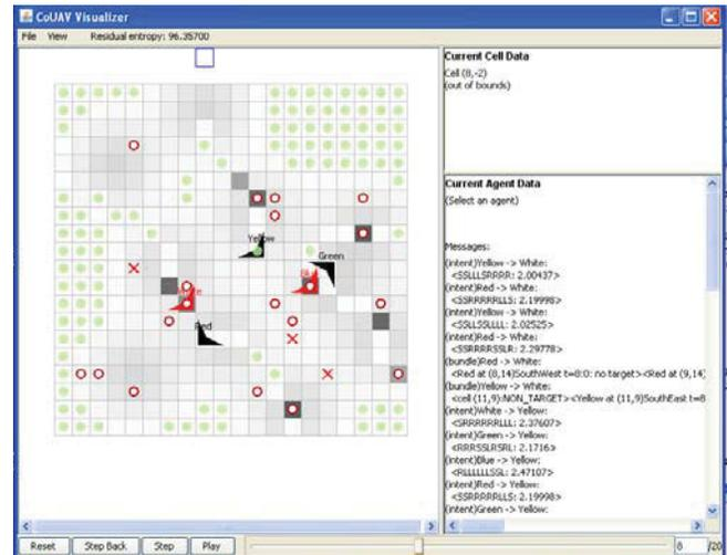
**Figure 5.** Cell occupancy probability distribution represented by different color shades. Ring symbols ('o') indicate real target locations to be discovered by team members. The darker the cell shade, the stronger the occupancy belief. Filled circles correspond to cells confirmed with certainty (red: positive, green: negative).
