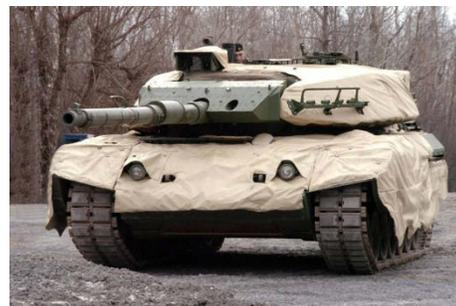
Figure 1: Heat shield on the Coyote light armoured vehicle (top) and the Leopard tank (bottom).
