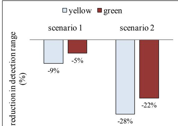
Figure 5: Visual spectrum percentage reduction in detection range for two sample scenarios. The green colouration of the electro-chromic cells improves the performance of the adaptive camouflage vehicle in the observed vegetated desert environment.
