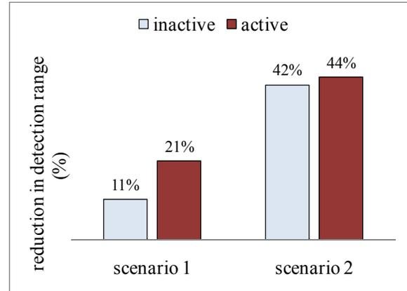
*Figure 4: Thermal infrared spectrum percentage reduction in detection range for two sample scenarios. The heating of the panels improves the performance of the camouflaged vehicle, increasing the percentage reduction of detection range as compared to the reference vehicle.*
