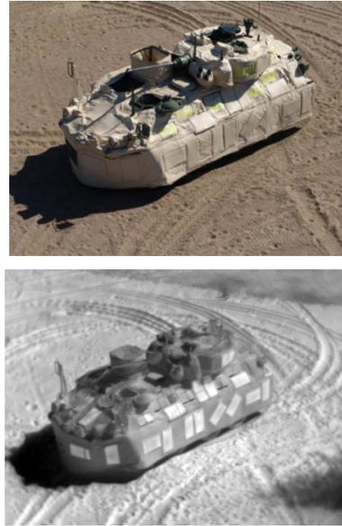
Figure 2: Heating patches in the visual (top) and infrared (bottom) bandwidths.
