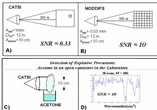
Figure 3: Evaluation of SNR for a MoDDIFS-type sensor based on SNR derived for CATSI.
