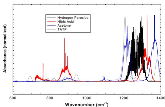
Figure 2: Absorbance spectra for vapours of important explosives and precursors.
