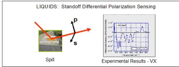
Figure 4: Differential polarization sensing scenario (left) and the resulting differential polarization spectrum showing the presence of VX.
