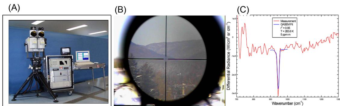
Figure 1: (A) Photograph of the CATSI instrument mounted on a tripod, (B) view of the 5.7-km long path facing towards the laboratory that contains the source, and (C) detection/identification of SF<sub>6</sub> at a distance of 5.7 km from the CATSI receiver.
