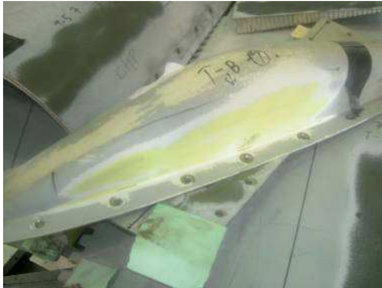
Figure 2: Stripped part showing selective removal of polyurethane topcoat leaving epoxy primer intact
