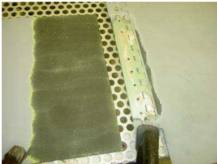
Figure 3: Graphite Epoxy panel showing no signs of fibre damage with complete paint removal.
