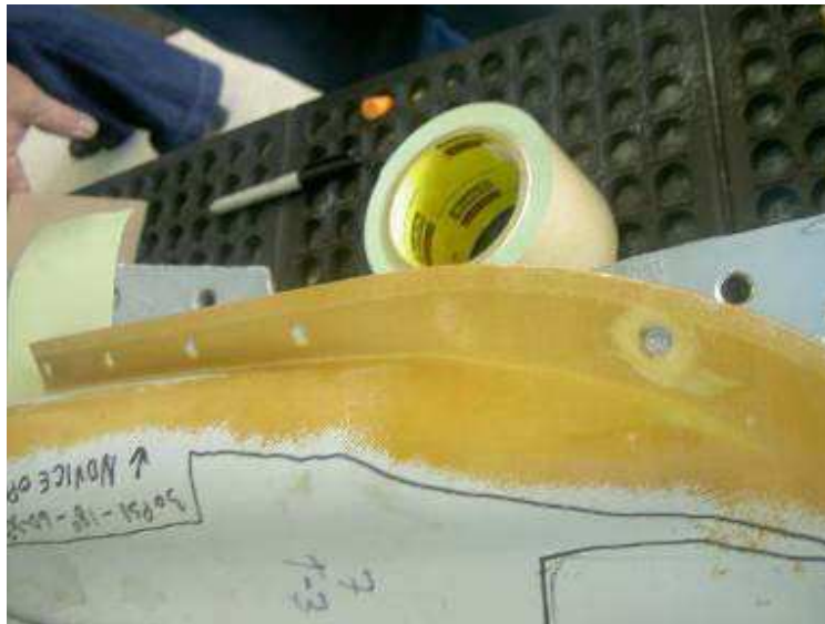
Figure 4: Stripped fibreglass part showing removal of coating and no fibre or fastener hole damage.
