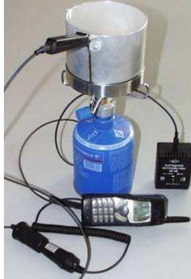
**Figure 13. A small thermoelectric battery charger that runs on the heat from a camp stove (Kryotherm).**
