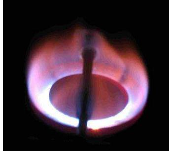
**Figure 8 Main burner of the stove in Fig. 1. Note the orange colour of the flame.**
