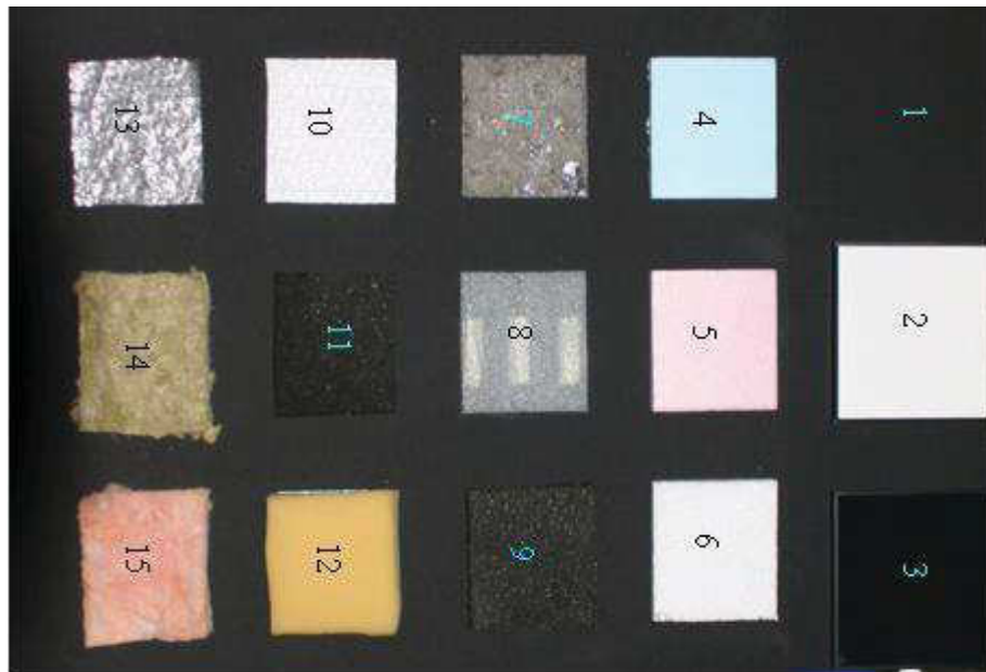
Figure 1c. For each panel type there is three permanent targets always on the top of the board. They are: black board (#1), 99% reflectivity Spectralon (#2) and 2% reflectivity Spectralon (#3). The dimensions of the Spectralons are 12cm x 12cm and the other subtargets 10cm x 10cm.
