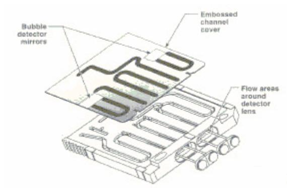
*Figure 12: RAPTOR cassette with 4 fiber optic probes*
