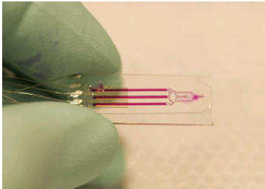
**Figure 11: Three channel Interdigitated Ultramicroelectrode Microfluidics Biosensor (from <http://www.ibi.cc/microfluidics.htm>)**
