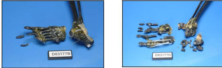
**Figure 4. Injury to FSL with standoff of 175 mm (left) and 125 mm (right)**
