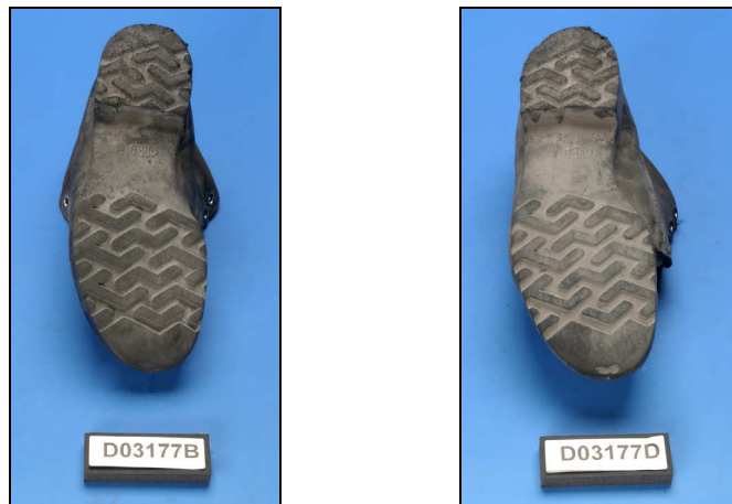
Figure 5. Boot damage with standoff of 175 mm (left) and 125 mm (right)
