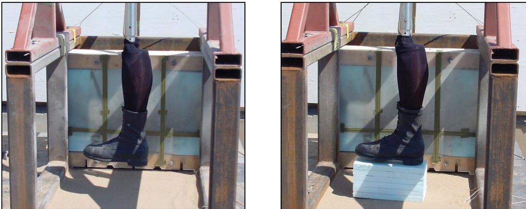
**Figure 1. Setup to study the effect of standoff on the level of injury; (left) with an air gap and (right) with Styrofoam<sup>®</sup> inserted.**
