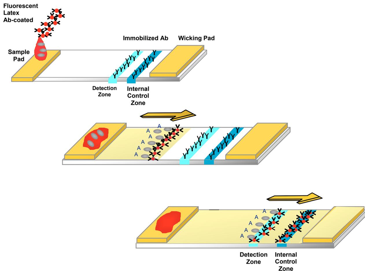
Figure 2. Diagrammatic representation of the principle of operation of the RAMP™ system (reproduced courtesy of W. Radvak, Response Biomedical Corp.)
