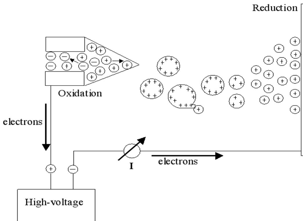
Figure 1: Schematic diagram of the electrospray ionization process.
