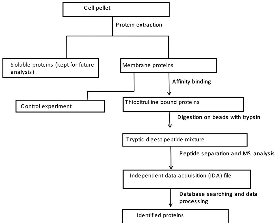
*Figure 3: A flow chart of the chemical proteomics and LC-MS process.*
