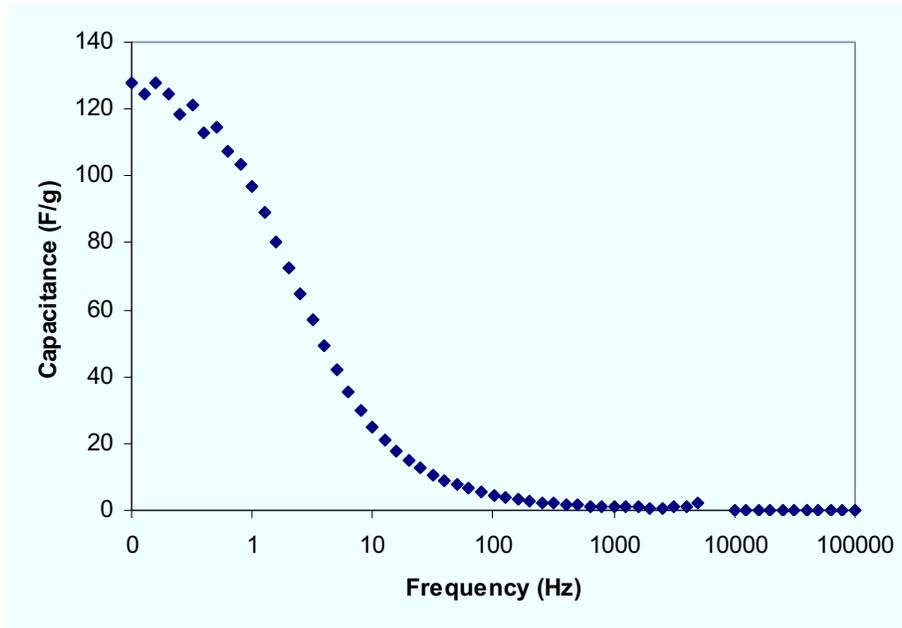
Figure 12: Capacitance versus Frequency Plot for PAni-2NSA/MWCNT.
