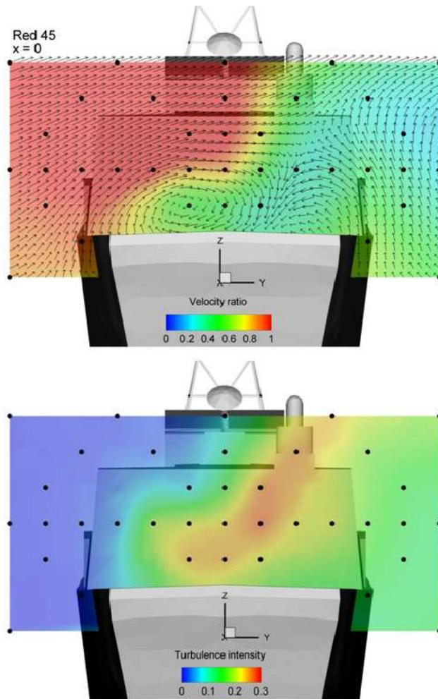
**Figure 5. Contours of velocity ratio and turbulence intensity of the time-averaged flow field in the ship coordinate system at  $x=0$  for Red45 wind. Black dots represent the locations of the virtual probes.**
