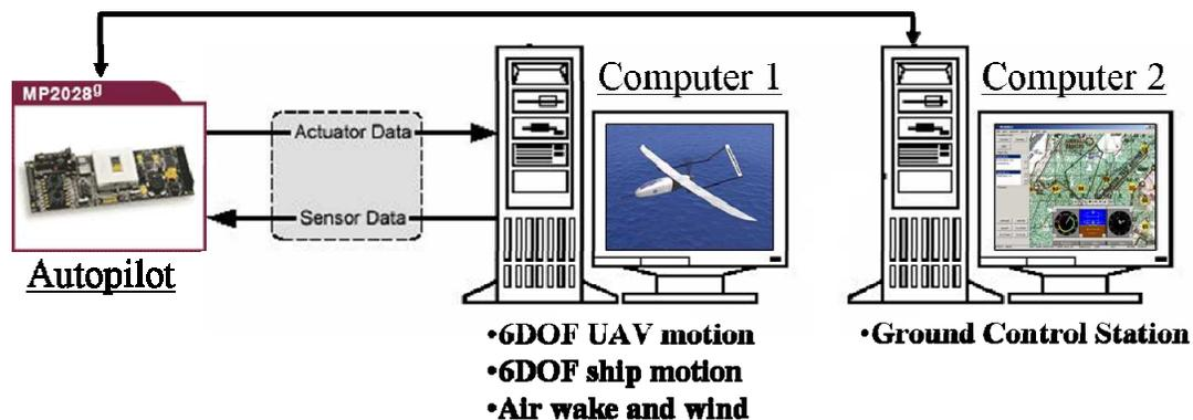
Figure 6. Hardware-in-the-loop simulation test bed.
