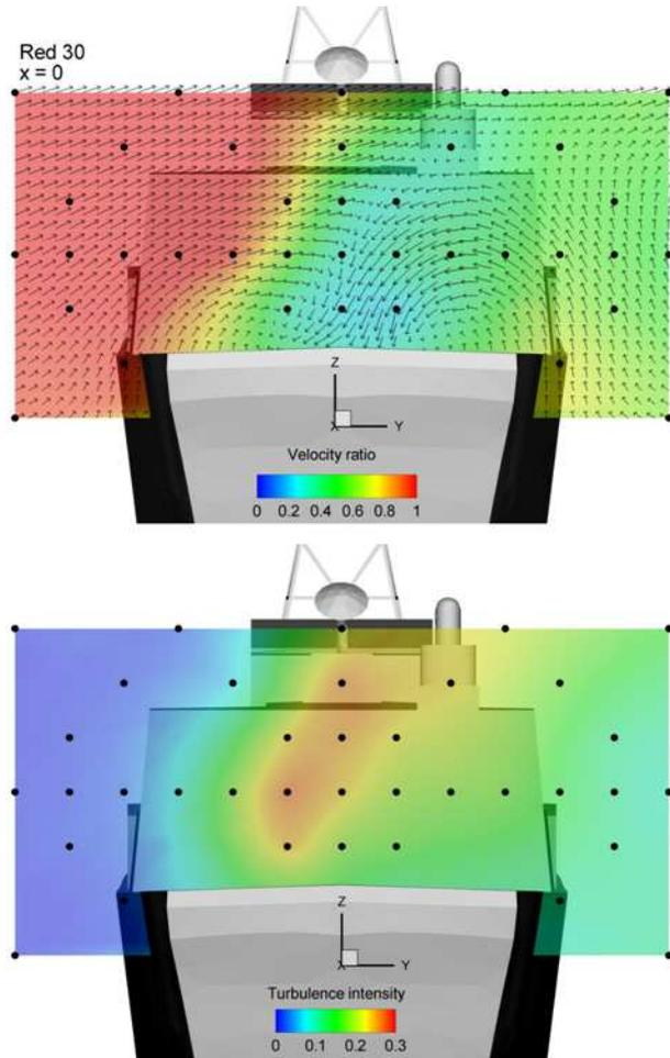
**Figure 4. Contours of velocity ratio and turbulence intensity of the time-averaged flow field in the ship coordinate system at  $x=0$  for Red30 wind. Black dots represent the locations of the virtual probes.**
