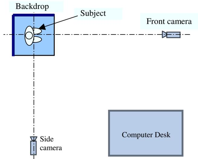
**Figure 1** Plan view of automated measurement set-up.
