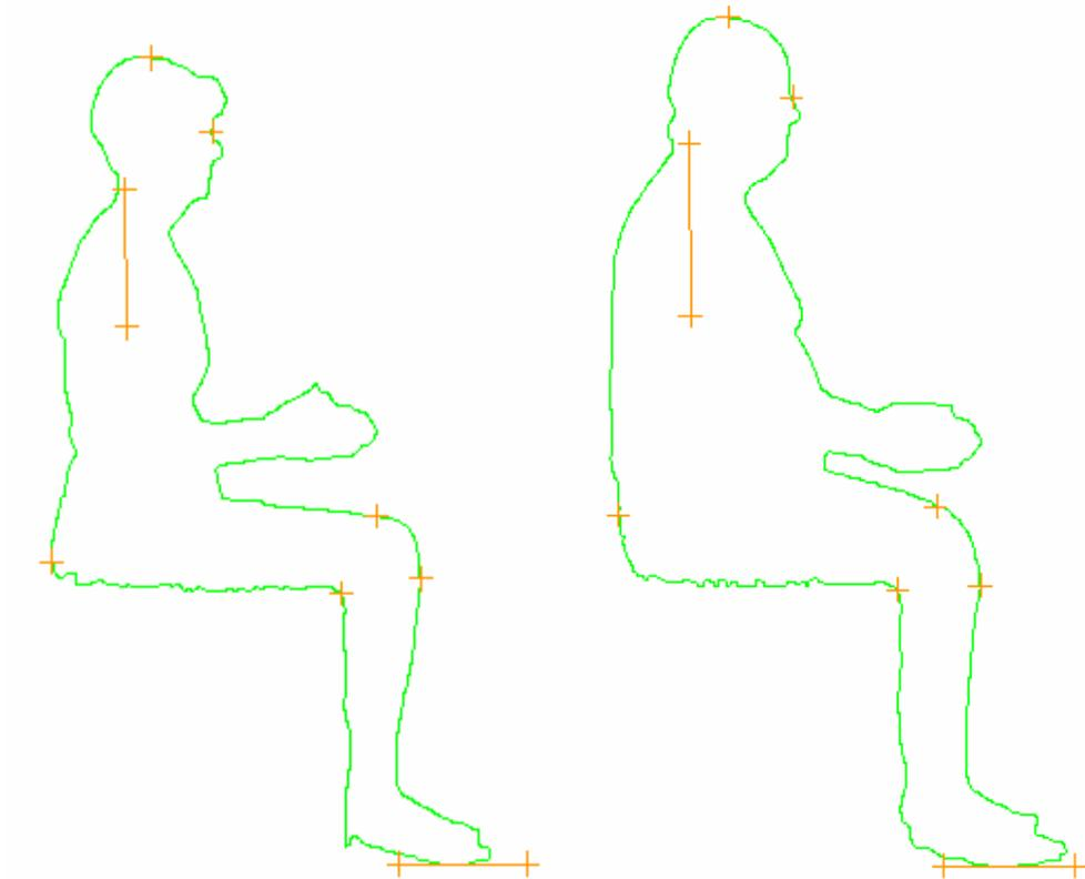
***Figure 9 Different cases in automated knee landmarking.***
