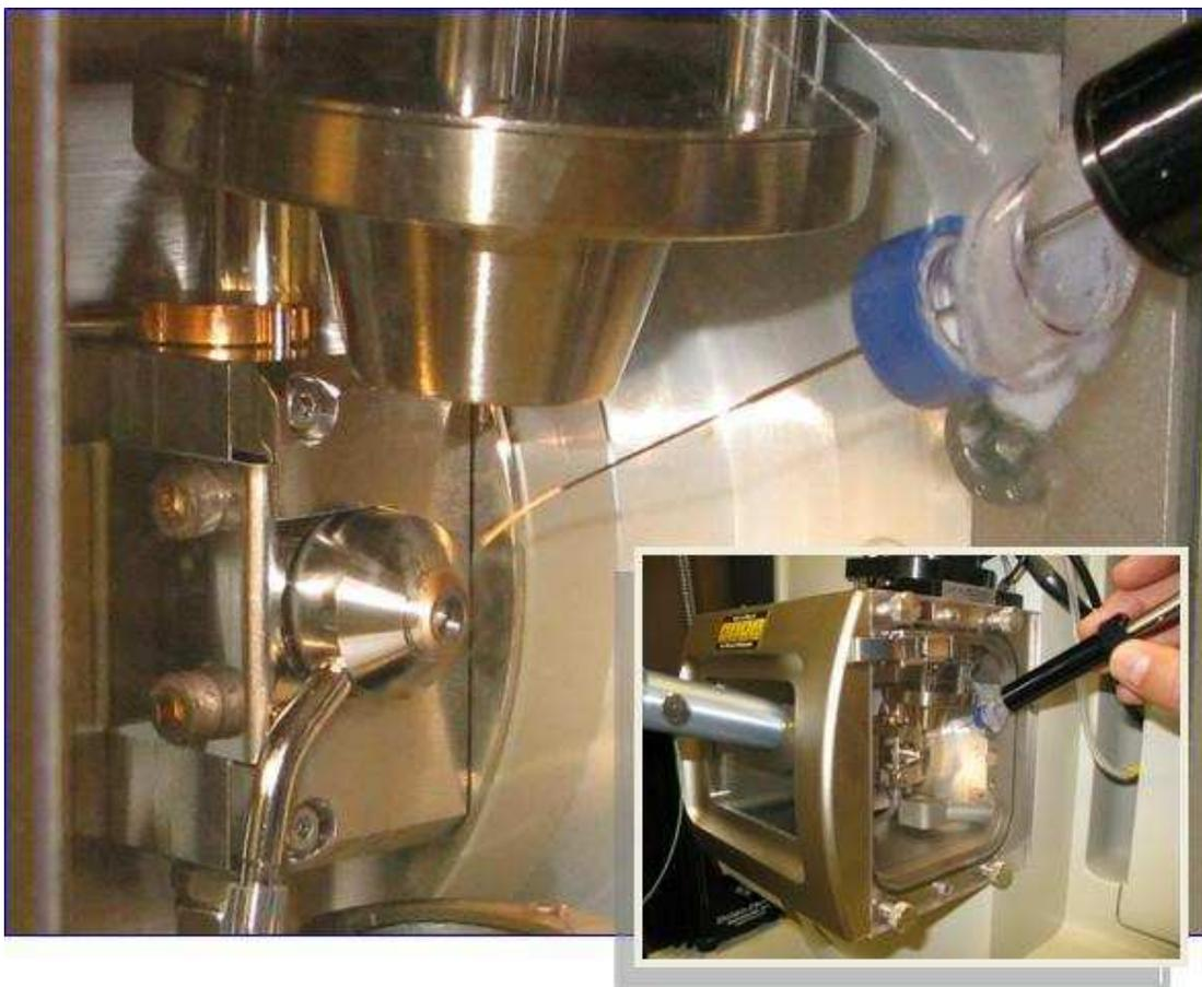
*Figure 1: DESI analysis of a SPME fiber in the Z-spray source of the Synapt HDMS (Inset: full view).*
