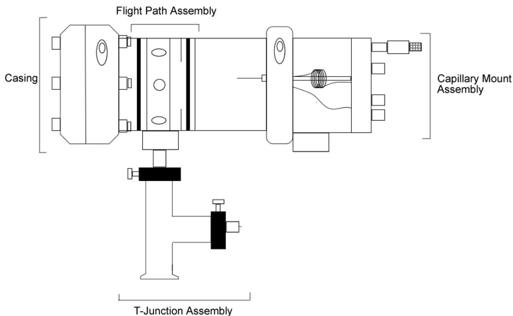
**Figure 1.1:** Side profile of the apparatus. The casing end is hereafter referred to as the front end, and the capillary mount assembly end is referred to as the rear end. Note that this is merely a simplified representation of the apparatus, and is not to scale.
