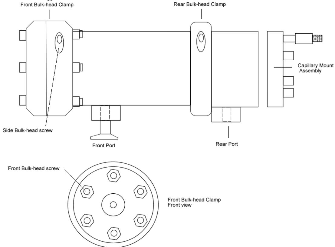
**Figure 1.2:** Plexiglass casing with its attached ports and clamps.
