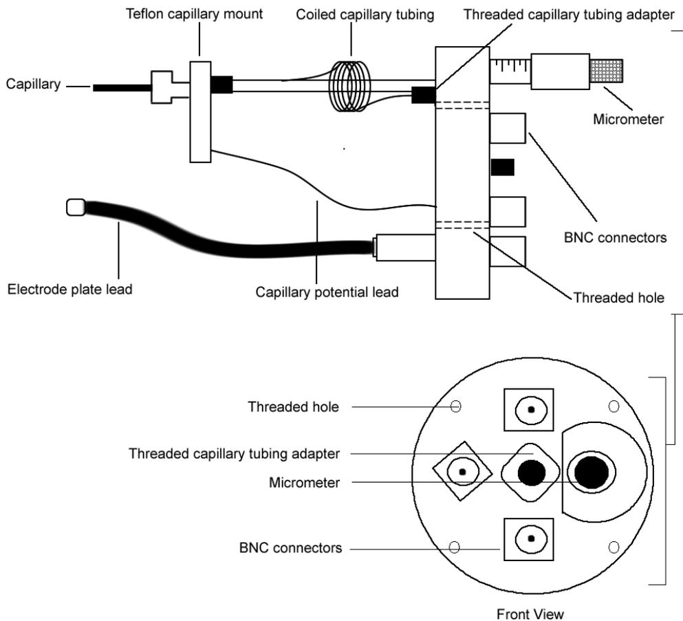
**Figure 1.3:** Capillary mount assembly detailed view
