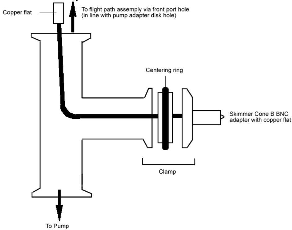
**Figure 1.5:** Cross section of the T-junction assembly; a 4-way junction can also be used.
