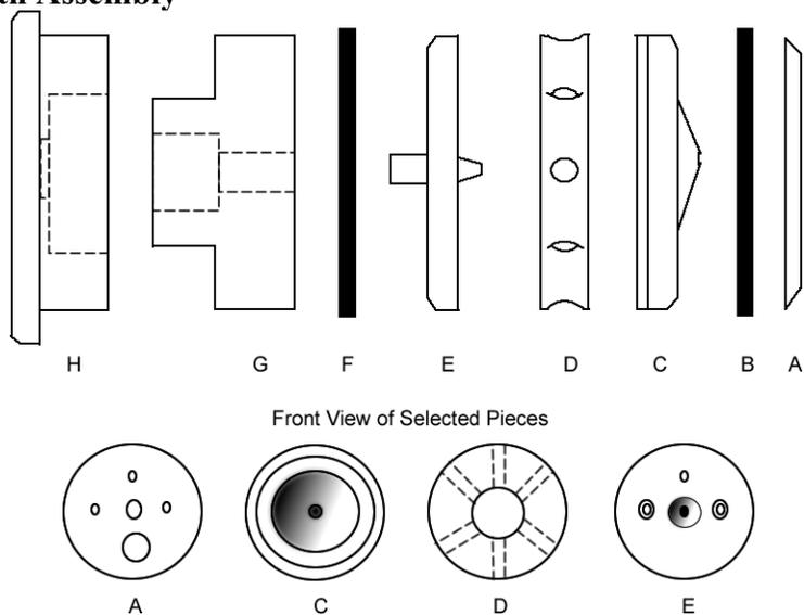
**Figure 1.4:** Flight path assembly pieces in the order they are placed inside the apparatus.
