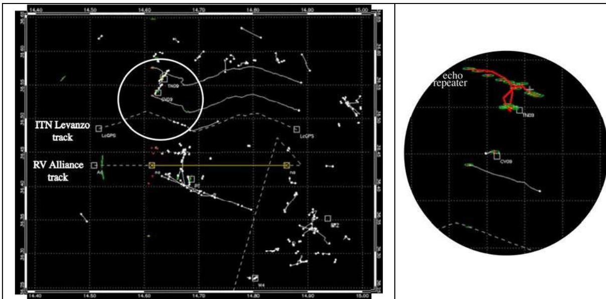
*Figure 5. Sample of ITAC tracker output. The east-west lines to the north of Levanzo's track (left panel) are detections of the echo-repeater signals. The circled area, expanded in the right panel, shows tracker error (loop) that results from detections from the Campo Vega tending tanker. Note that only tracks (not individual detections) are displayed.*
