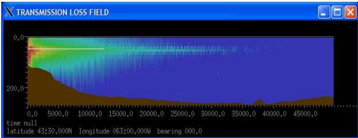
Figure 6. Transmission Loss vs. Range and Depth Display
