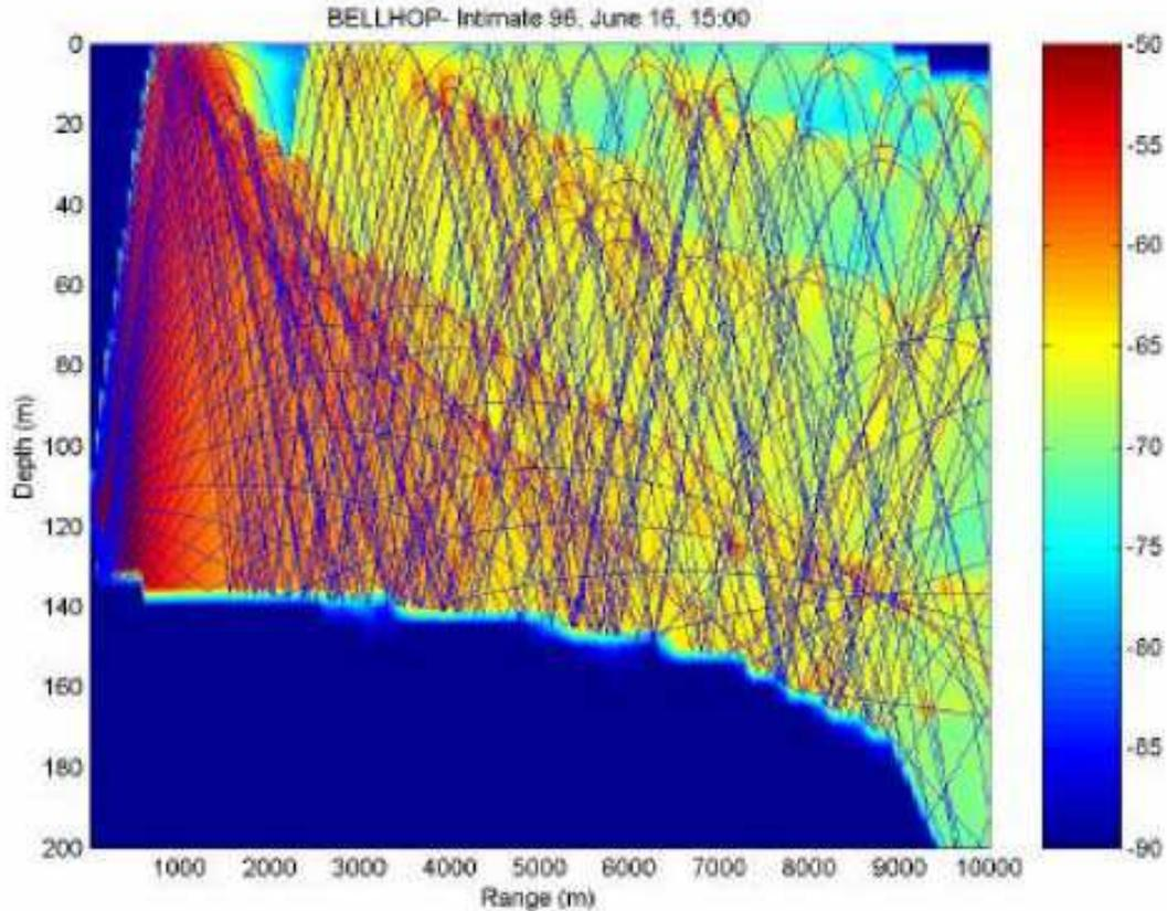
*Figure 9. Combined Ray-Plot and Propagation Loss Display*
