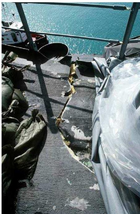
**Figure 3-3.** One of the cracks in the USS Princeton's hull as a result of the mine it hit.
