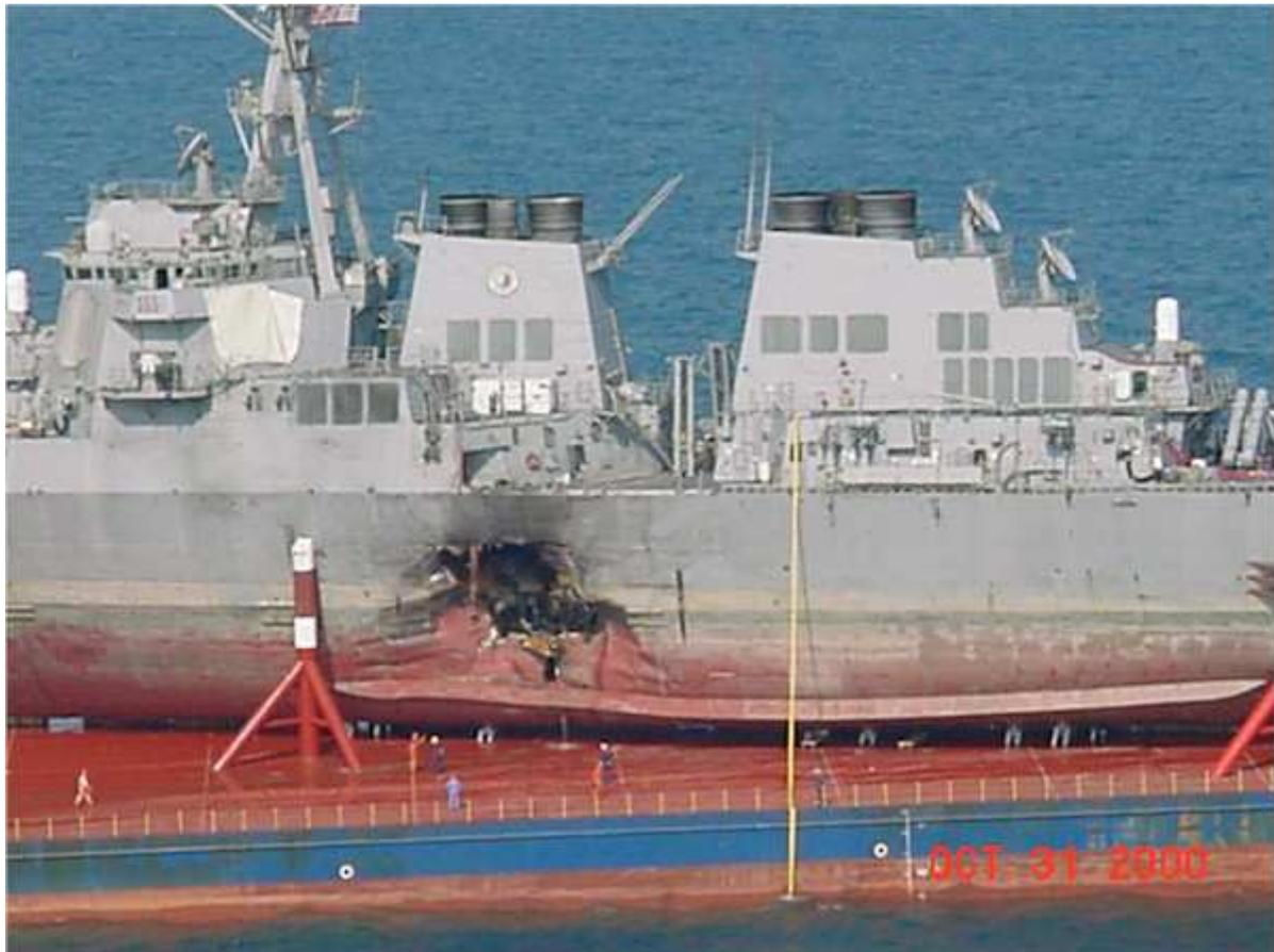
**Figure 3-2.** A close-up of the damage inflicted on the USS Cole. For scale purposes, note the size of the sailors in the foreground.
