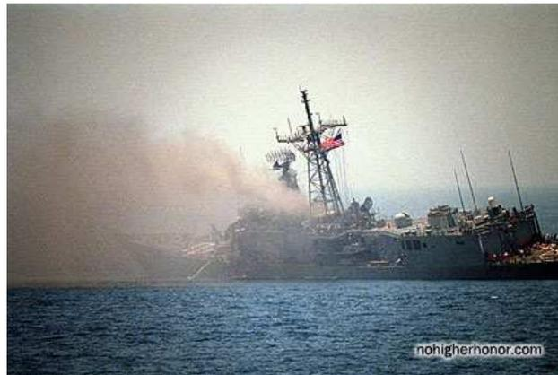
**Figure 3-4.** The USS Stark, severely listing to port as a result of flooding.
